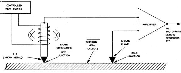
FIG. 3 Typical Circuit used in Thermoelectric Sorting Instruments
