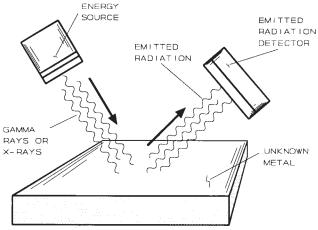
FIG. 1 X-Ray Fluorescence Spectrometry
