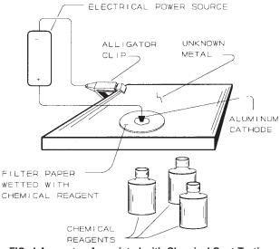
FIG. 4 Apparatus Associated with Chemical Spot Testing
