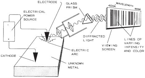
FIG. 2 Optical Emission Spectrometry
