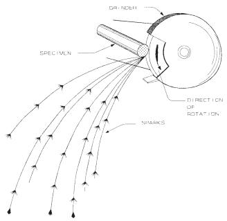
FIG. 5 Typical Spark Test
