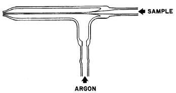
FIG. 2 Concentric Glass Nebulizer (CGN)<sup>4</sup>
