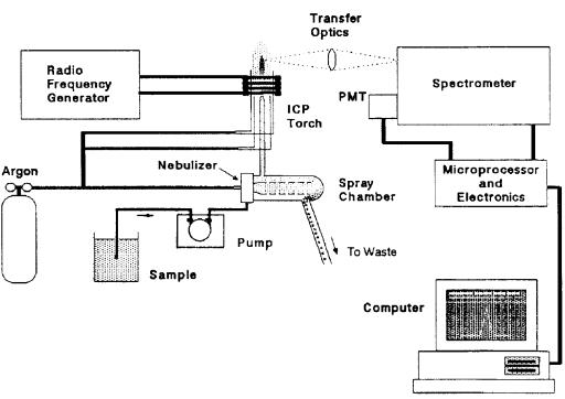
FIG. 1 Components of Inductively Coupled Plasma<sup>4</sup>
