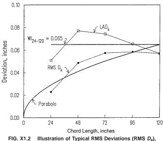
FIG. X1.2 Illustration of Typical RMS Deviations (RMS  $D_k$ ), Length-Adjusted Deviations ( $LAD_k$ ), and Waviness Index (*WI*)
