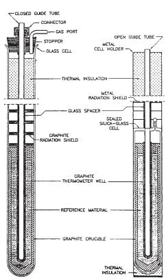
FIG. 3 Examples of Freezing-Point Cells
