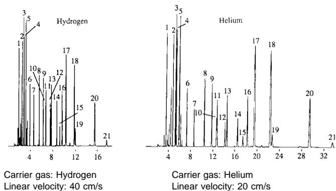
NOTE 1—Fig. 2 shows that the resolution is similar but the analysis time is reduced by 50 % when comparing hydrogen to helium in an isothermal analysis using optimum flow velocities.
