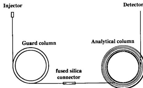
NOTE 1—A guard column protects the analytical column from damage by nonvolatile residue, particulates, or derivatization.
