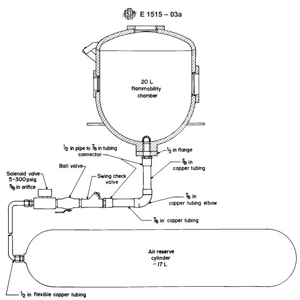
FIG. X1.3 Schematic of Bureau of Mines 20-L Chamber, Showing Air Reserve Cylinder and Dispersion Plumbing
