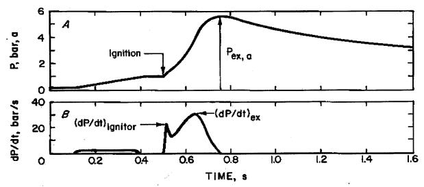
FIG. 2 Typical Recorder Tracings for a Moderate Dust Deflagration in a 20-L Chamber, using a 2500 J Ignitor
