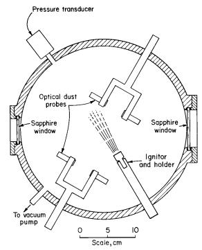
FIG. X1.2 Horizontal Cross Section of Bureau of Mines 20-L Chamber
