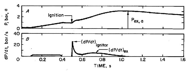
FIG. 1 Typical Recorder Tracings for a Weak Dust Deflagration in a 20-L Chamber, using a 2500 J Ignitor
