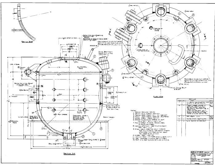
FIG. X1.4 Machine Drawings of Bureau of Mines 20-L Chamber
