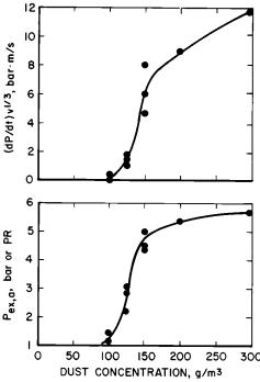
FIG. 3 Explosibility Test Data as a Function of Concentration for a Typical Dust in a 20-L Chamber, using a 2500 J Ignitor
