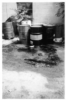
FIG. X2.12 Surface Staining from Improper Drum Storage
