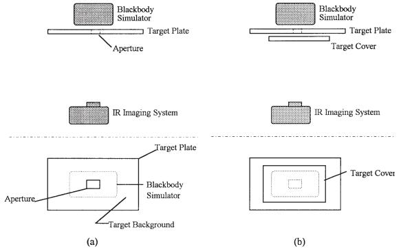
FIG. 1 Schematic of NETD Test Configuration; (a) When Measuring Signal and (b) When Measuring Noise
