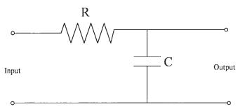
FIG. 2 Circuit Diagram of Standard Reference Filter
