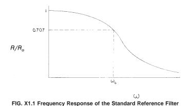
angular frequency ( $\omega = 2\pi f$ ). The frequency at which  $R/R_o$  equals 0.707 is the characteristic frequency, given by:
