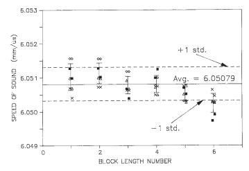
Note 1—Four different ultrasonic transducers were used and are indicated by different symbols. Two sets of values were taken for each transducer. "I" bars are estimated error limits for all the data of one path length as determined from the standard deviation of each set. The average value and the standard deviation of the total data set are shown.
