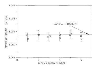
Note 1—15 MHz transducer with a fast rise time was used. Each data point represents many data points on the same value. Precision was limited by the least count and by the setability of the measurement equipment. Error "I" bars are determined by plus or minus the setability. Average is for the total set. This demonstrates a definite "pass" to the necessary criterion of speed of sound = constant.
