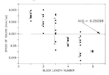
Note 1—The error "I" bars are determined from the average and the standard deviation of each path length set. The average is for the total set.
