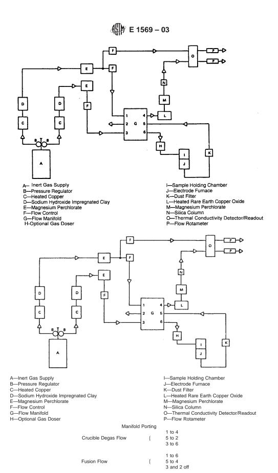
FIG. 1 Apparatus for the Determination of Oxygen by the Inert Gas Fusion—Thermal Conductivity Method
