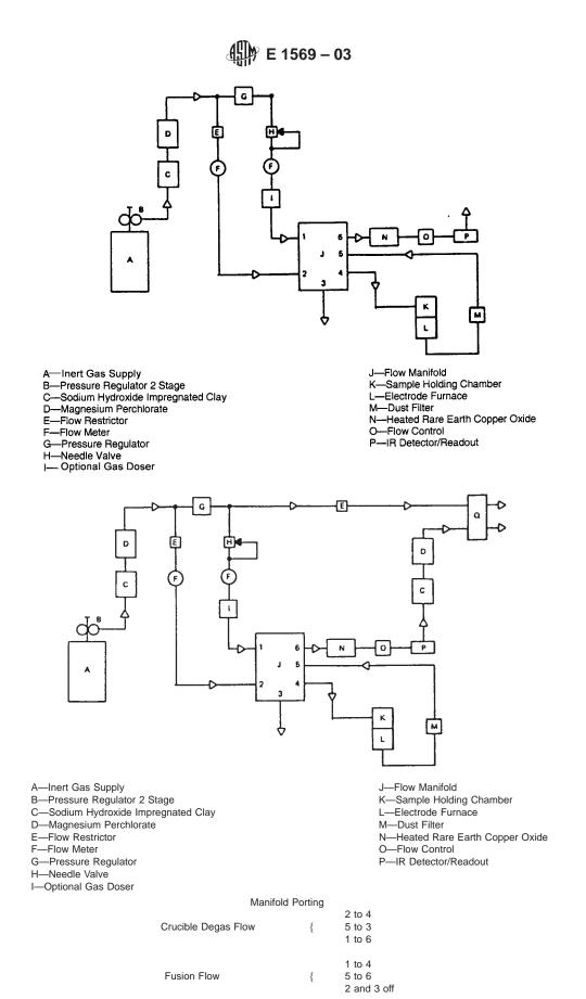
FIG. 2 Apparatus for the Determination of Oxygen by the Inert Gas Fusion—Infrared Absorption Method
