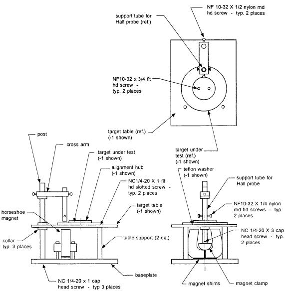
FIG. X1.1 Magnetic Test Fixture—Assay
