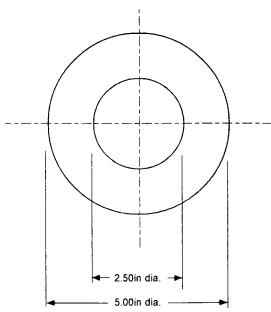
FIG. X1.9 - 1 TFE-Fluorocarbon Washer
