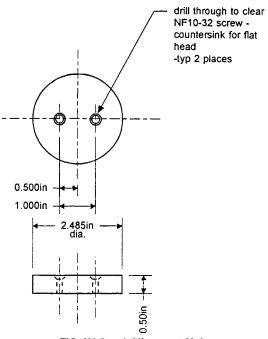
FIG. X1.8 - 1 Alignment Hub
