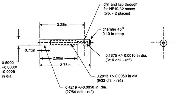
FIG. X1.10 Probe Support Tube
