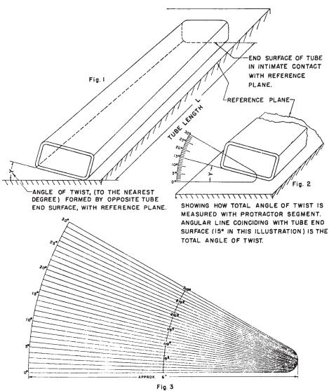
SHOWING TRANSPARENT PLASTIC PROTRACTOR SEGMENT RECOMMENDED FOR DETERMINING TOTAL ANGLE OF TWIST.
