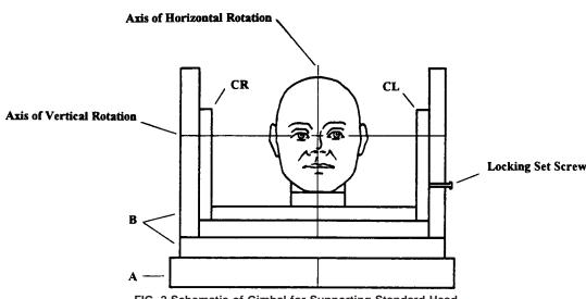
FIG. 2 Schematic of Gimbal for Supporting Standard Head
