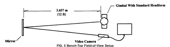
response of the two eyes. The gimbal then is rotated to determine the horizontal and vertical extreme angles of view in all four directions along which the appropriate corneas can be seen monocularly.
