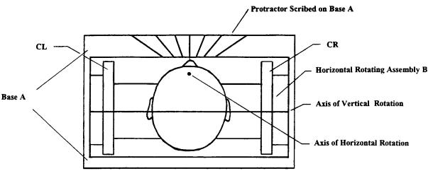
FIG. 4 Top View Showing Base for Horizontal Rotation
