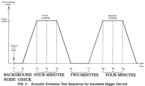
load shall be 150 % of its rated capacity. Where applicable the actual loadline shall be used.
