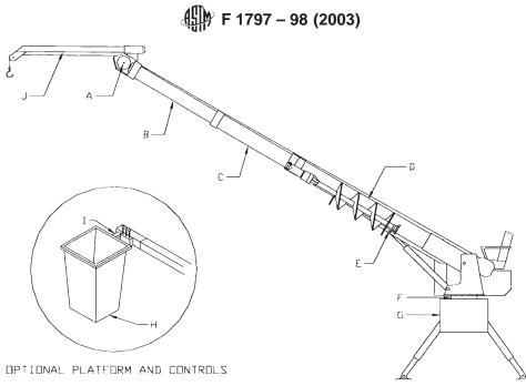
FIG. 1 Insulated Digger Derrick Nomenclature
