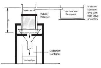
Note 1—The hydraulic head (h) is measured from the bottom of the soil column to the water level above the soil.
