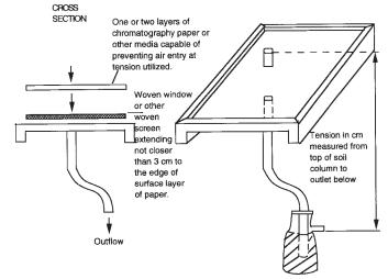
FIG. 2 Suggested Tension Apparatus Capable of Extracting Water out of the Soil Cores
