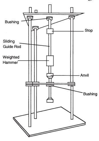
NOTE 1—It has been found that 15 drops of the hammer from a height of 12 in. (as measured from the bottom of the weight to the top of the anvil) will produce a degree of compaction comparable to a severely compacted putting green, provided the soil contains moisture approximating field capacity.
