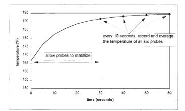
FIG. 2 Timing of Temperature Measurement After Probes are Placed on Cooked Pizza
