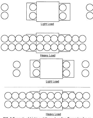
FIG. 3 Example of Light and Heavy Loading Scenarios for an Oven With a 2 ft Conveyor Width and a 3 ft Cavity Length
