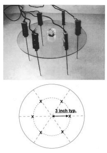
NOTE 1—The structure shown in the above photograph can be gently set on top of the pizza during cook-time determination with just enough force to penetrate the cheese but not enough to push the probes beyond the sauce-crust interface. Because the sauce migrates into the crust during cooking, it is relatively easy to remain in the sauce-crust interface during temperature measurement.
