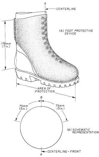
FIG. 2 Footwear With Front Closure Device
