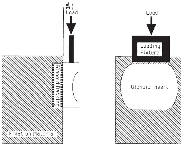
FIG. 2 Schematic of Static Glenoid Locking Strength Anterior to Posterior Direction
