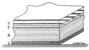
Note 1—(A) Poly(methyl methacrylate) sheet,  $0.25\pm0.03$ -in. (6  $\pm$  0.1-mm) thickness; (B) AC exterior glue fir plywood sheet,  $0.75\pm0.08$  in. (19  $\pm$  0.2 mm) or greater in thickness; (C) polypropylene microfoam sheet;  $0.7\pm0.01$ -lb/ft³ (11  $\pm$  0.2-kg/m³) density and  $0.13\pm0.01$ -in. (3  $\pm$  0.03-mm) thickness; and (D) glass/tempered sheet,  $0.38\pm0.04$ -in. (10  $\pm$  0.1-mm) thickness.
