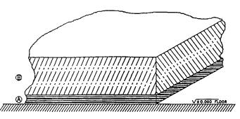
Note 1—(A) Poly(methyl methacrylate) sheet, 0.25  $\pm$  0.03-in. (6  $\pm$  0.1-mm) thickness; and (B) AC exterior glue fir plywood sheet, 0.75  $\pm$  0.08 in. (19  $\pm$  0.2 mm) or greater in thickness.
