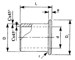
FIG. X1.2 Standard Flange Bearing
