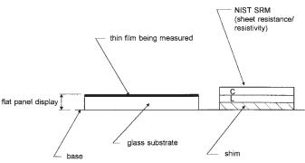
FIG. 3 Specimen Positioning Between Transducers
