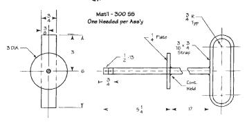
Note 1—Dimensions in inches. FIG. A1.5 Loading System, Part T-4, Handle
