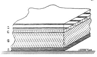
Note 1—(A) Poly(methyl methacrylate) sheet, 0.25  $\pm$  0.03-in. (6  $\pm$  0.1-mm) thickness; (B) AC exterior glue fir plywood sheet, 0.75  $\pm$  0.08 in. (19  $\pm$  0.2 mm) or greater in thickness; (C) polypropylene microfoam sheet; 0.7  $\pm$  0.01-lb/ft³ (11  $\pm$  0.2-kg/m³) density and 0.13  $\pm$  0.01-in. (3  $\pm$  0.03-mm) thickness; and (D) glass/tempered sheet, 0.38  $\pm$  0.04-in. (10  $\pm$  0.1-mm) thickness.
