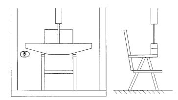
Note 1—(A) = block and (B) = application of block to chair. FIG. 8 250-lb (114-kg) Arm Testing Block
