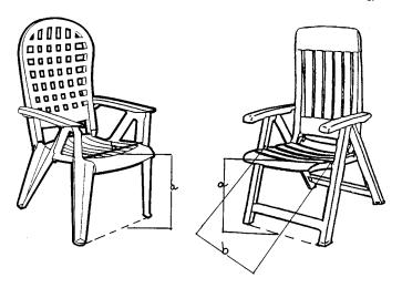
Note 1—(a) Seat height with the seat and back in the most upright position; and (b) seat width.
