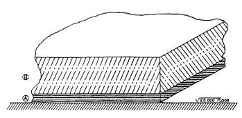
Note 1—(A) Poly(methoyl methoacrylate) sheet, 0.25  $\pm$  0.03-in. (6  $\pm$  0.1-mm) thickness; and (B) AC exterior glue fir plywood sheet, 0.75  $\pm$  0.08 in. (19  $\pm$  0.2 mm) or greater in thickness.
