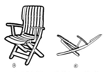
Note 1—(A) Chair with the seat and back in the most upright position; and (B) chair with the back resting in the furthest reclining position and arms locked in the furthest reclining position.
