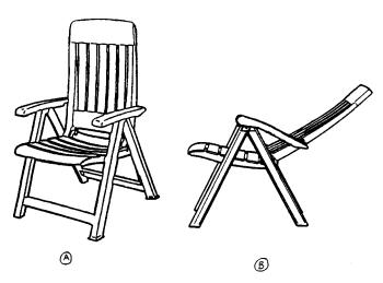
Note 1—(A) Chair with the seat and back in the most upright position; and (B) chair with the back resting in the furthest reclining position and arms locked in the furthest reclining position.
