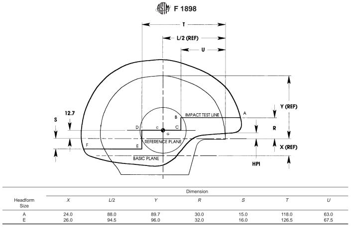
NOTE 1—This test line drawing shows test lines on helmet rather than on headform and uses dimensional nomenclature R, S, T, U as in other drawings (formerly a, b, c,...). The position of the lines on this drawing has not changed except that they are a bit more stringent because of the angle of projection from the c/g, which is the center of the ball about which the headform pivots to align an impact site with the anvil.
