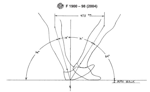
FIG. 2 Typical Ranges of Motion During Ground Contact During Walking at 3.2 kph (2.0 mph)
