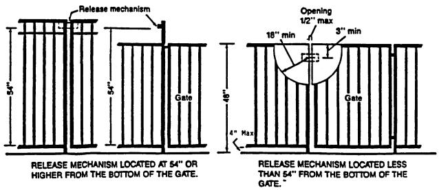
FIG. 4 Latch Release Mechanism
