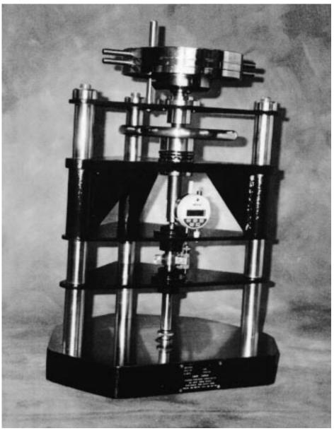
FIG. 1 Apparatus for Measuring Indentation and Residual Indentation
