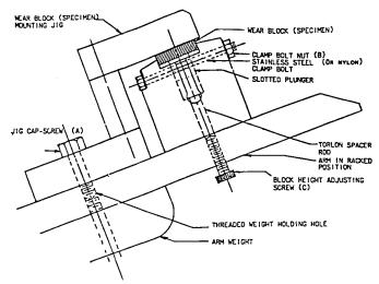
FIG. 6 Wear Block/Wear Specimen Alignment Jig
