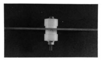
FIG. 4 Multiple Crevice Assembly with Sheet Specimen
