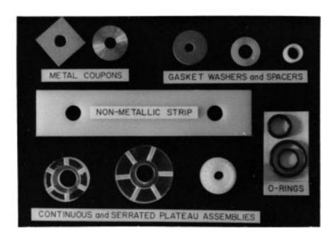
NOTE 1—Various crevice former designs utilized in laboratory and field test crevice-corrosion studies. Severity of the test may vary as a function of crevice geometry, that is, size of the crevice former and degree of tightness
