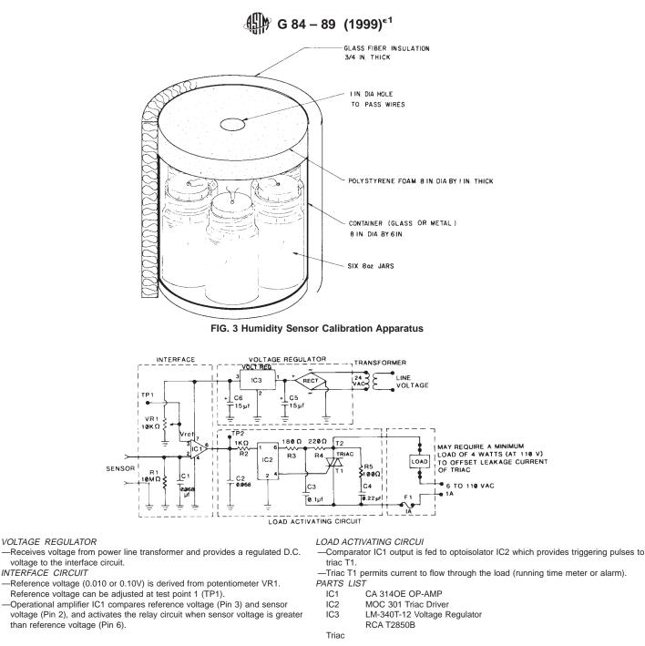
FIG. 4 Line Powered Wetness Detector
