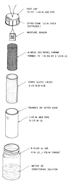
FIG. 2 Humidity Sensor Calibration Apparatus
