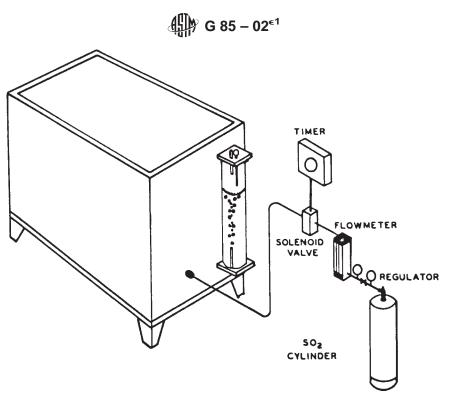
FIG. A4.1 Schematic of SO<sub>2</sub> Line into Salt Fog Cabinet
