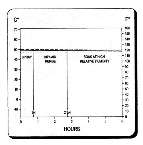
Note 1—Dashed chart lines indicate temperature tolerance limits. Note 2—Reprinted with permission.
