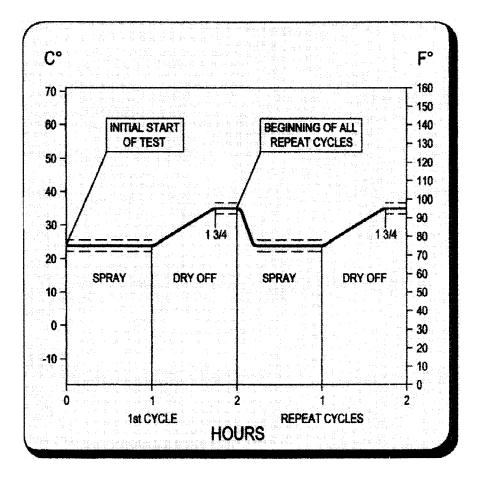
NOTE 1—Dashed chart lines indicate temperature tolerance limits. NOTE 2—Temperature changes illustrated are pictorial representations only and are not based on actual tests.
