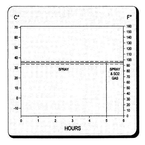
Note 1—Dashed chart lines indicate temperature tolerance limits. Note 2—Reprinted with permission. FIG. X4.1 Cyclic Salt/SO<sub>2</sub> Spray (Fog) Testing (Example A4.4.4.1)
