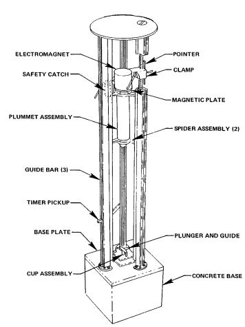
FIG. 1 Oxygen Impact Test Frame
