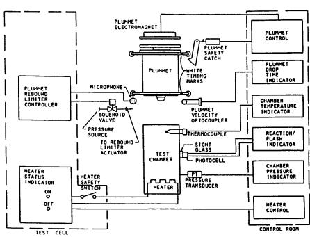
FIG. 9 Typical Instrumentation/Control Diagram for Pressurized LOX/GOX System
