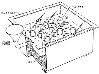
FIG. 6 Typical Sample Freezing Box
