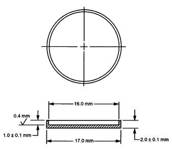
Note 1—Material: Type 347 stainless steel. Note 2—Break all sharp edges 0.19 mm.
