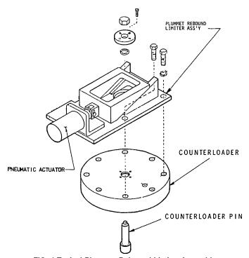
FIG. 4 Typical Plummet Rebound Limiter Assembly
