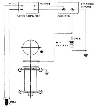
FIG. 13 Typical Free-Fall Timing Circuit
