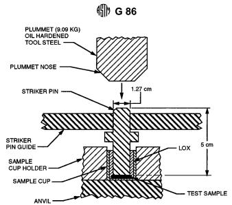
FIG. 12 LOX Impact Tester Sample Cup, Sample Cup Holder, Striker Pin, and Anvil Configuration
