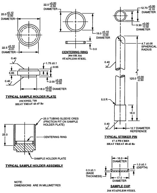
FIG. 14 Typical Test Chamber Internal Components
