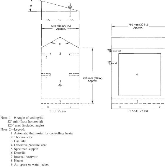
FIG. X1.1 Typical Moist SO<sub>2</sub> Test Chamber
