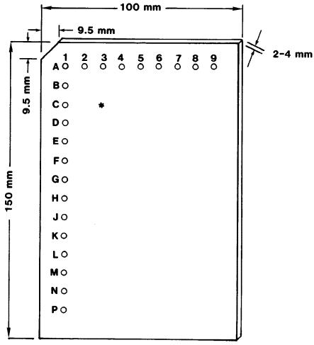
\* Template contains 126 drilled holes
