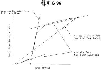
FIG. 3 Typical Plot of Metal Loss Versus Time
