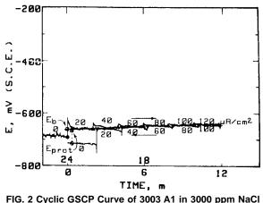
FIG. 2 Cyclic GSCP Curve of 3003 A1 in 3000 ppm NaCl (Taken from Ref. 7)
