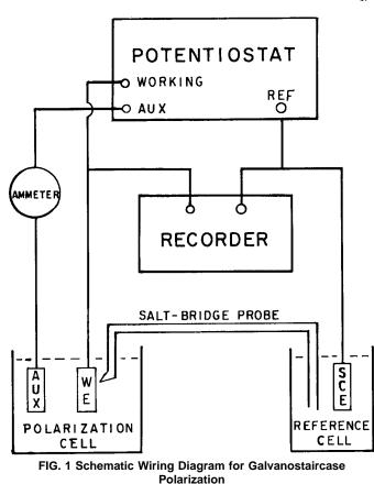
may be replaced by a plotter if the current staircase signal is generated with the aid of a computer. The current staircase may be generated manually (Note 2) but this is not recommended. The most convenient current staircase generators are found in recent commercial potentiostats where the software is available. The electrical equipment may be checked in accordance with the procedure in Practice G 59.
