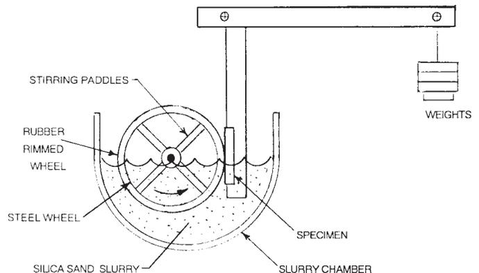
FIG. 1 Schematic Diagram of the Wear Test Apparatus
