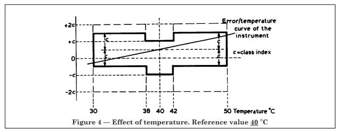
The solid boundary shown in Figure 5 represents the error limits within the nominal range of use expressed in multiples of the class index. The indication corresponding to any point within the effective range is only correct within a tolerance represented by a point within the boundary line, i.e.:
