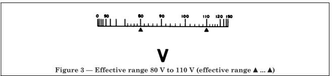
The limits of the effective range and the fiducial value are not dependent on the zero mark, which may be at either end of the scale, displaced within the scale, or non-existent.
