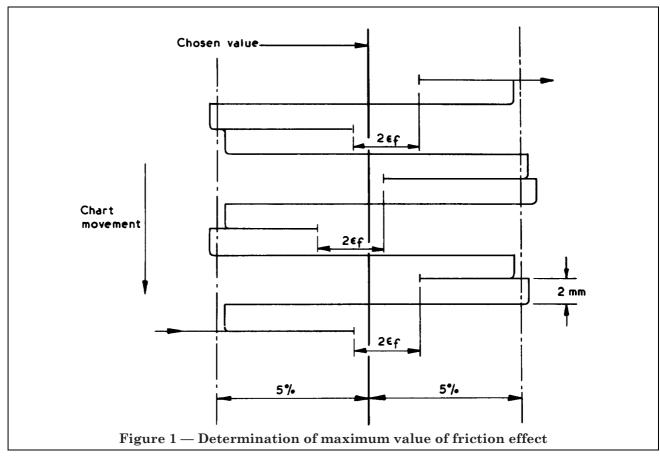
**9.2.2** The maximum value of friction effect determined according to **9.2.1** shall not exceed the limit which is specified by the manufacturer and marked on the instrument (symbol K-1 of Table 17).
