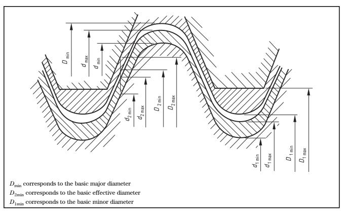
Figure 4 Example of effective diameter tolerance zones (Effective diameter tolerance zones for size 2 B.A. threads illustrated)
