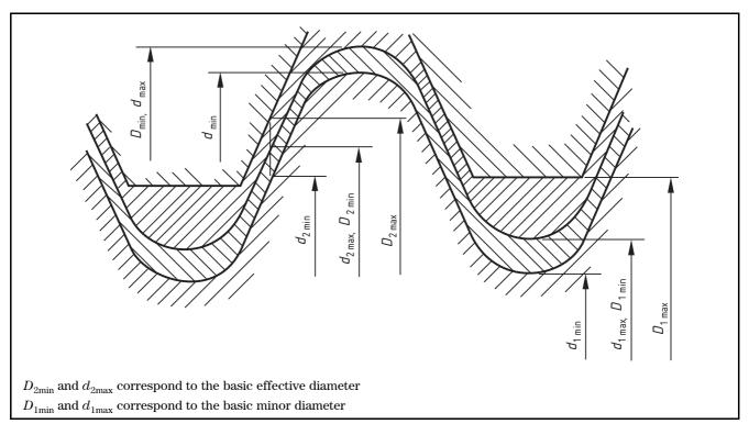
$\begin{tabular}{ll} Figure 3 & \textbf{Tolerance zones for a normal class external thread and an internal thread} \end{tabular}$
