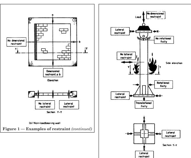
(c) Column pinned one end  ${f Figure 1-Examples of restraint}\ (continued)$
