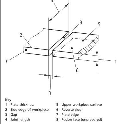
Figure 6 Preparation for butt weld between plates with raised edges
