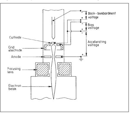
Figure 85 Diagrammatic representation of a back-bombarded gun
