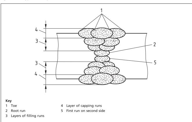
Figure 62 Typical example of multi-run fusion weld – Double V-butt weld
