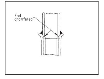
Figure 89 Diminishing bell butt joint
