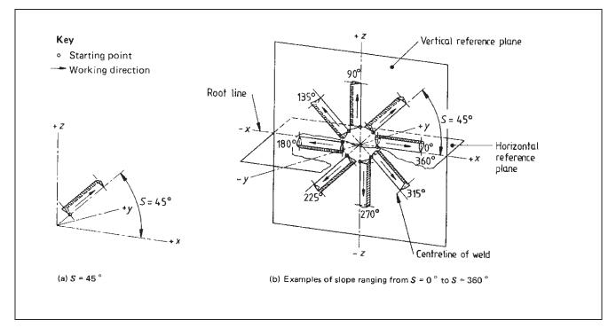
Figure 56 Schematic diagram of main welding positions
