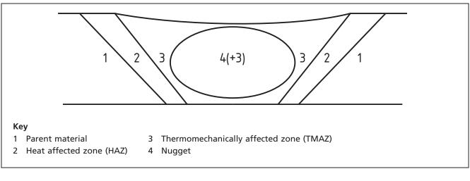
Cross-section of a friction stir weld
