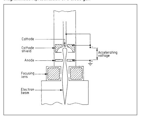
Figure 84 Diagrammatic representation of a triode gun
