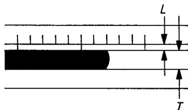
Figure 2 — Examples of graduation showing the position of the scale lines relative to the enlarged image of the mercury column where  $L$  is less than  $0.5 T$  (see 7.6)
