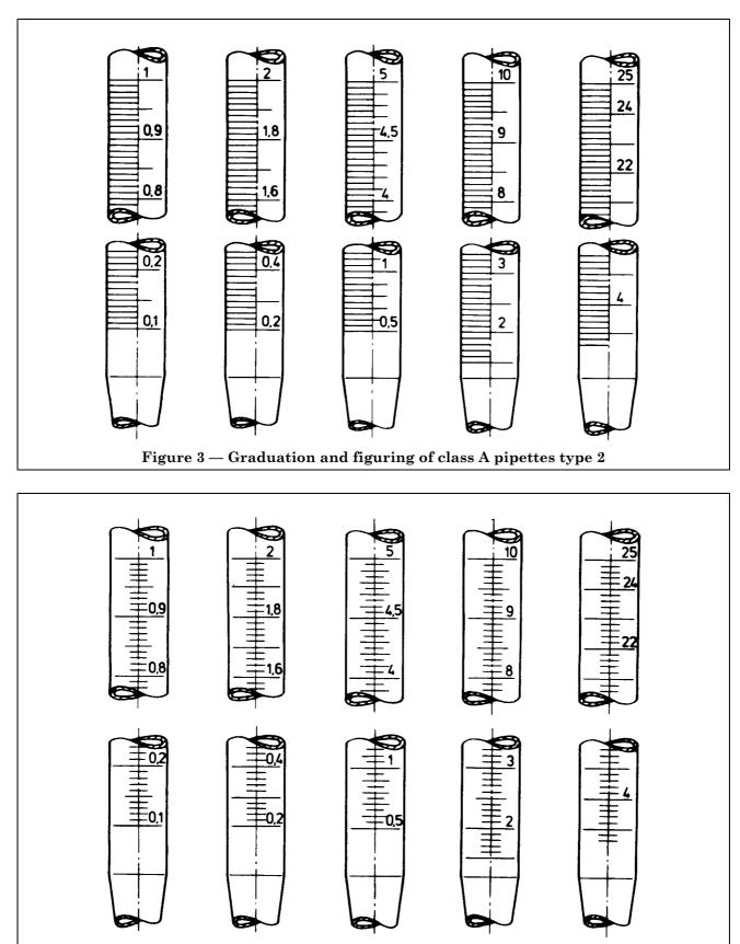
Figure 4 — Graduation and figuring of class B pipettes type 2
