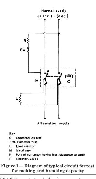
**5.2.5.2** The contactor shall make a current of  $7 \times$  full-load current at any convenient voltage without welding, and the current shall be interrupted by another device immediately after the contactor has closed. The test shall be repeated for 10 cycles at intervals not exceeding 2 min.
