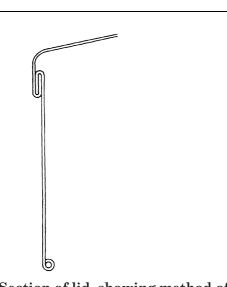
Figure 2 — Section of lid, showing method of seaming on flange, and form of internal bead
