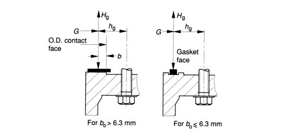
NOTE. The gasket seating width factors  $b_0$  and b shown apply only to flanged joints in which the gasket is contained entirely within the inner edges of the bolt holes.
