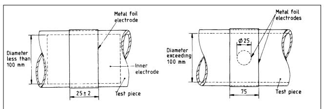
(a) Electrodes for tests on round tubes less than 100 mm diameter
