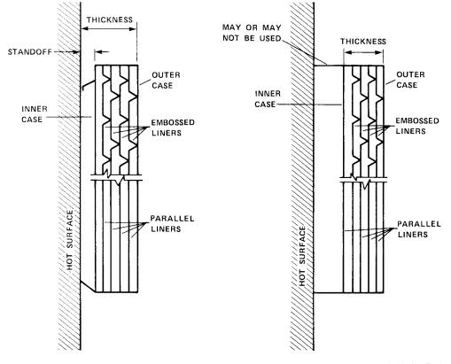
(a) Reflective Insulation Applied to Piping (b) Reflective Insulation Applied to Equipment FIG. 1 Illustration of Terms Relating to Prefabricated Reflective Insulation Systems not be made of aluminum or aluminum alloys. If components will be elevated to 1200°F (649°C) or higher, Type 300 series austenitic stainless steel should be used. Other materials and alloys are available for use over 1200°F (649°C).
