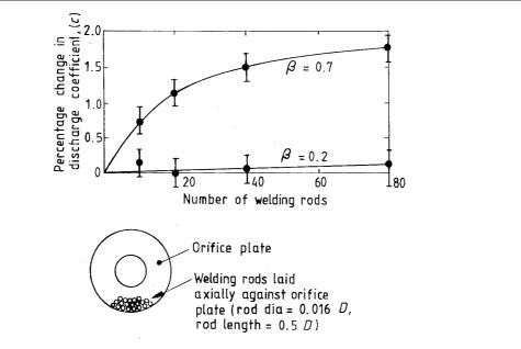
Figure 11. Effect of welding rods in meter tube
