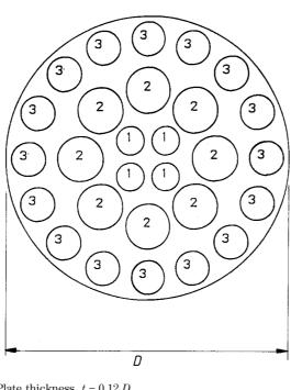
Plate thickness, t = 0.12 DHole diameter,  $d_1 = 0.10 D$ Hole diameter,  $d_2 = 0.16 D$ Hole diameter,  $d_3^2 = 0.12 D$
