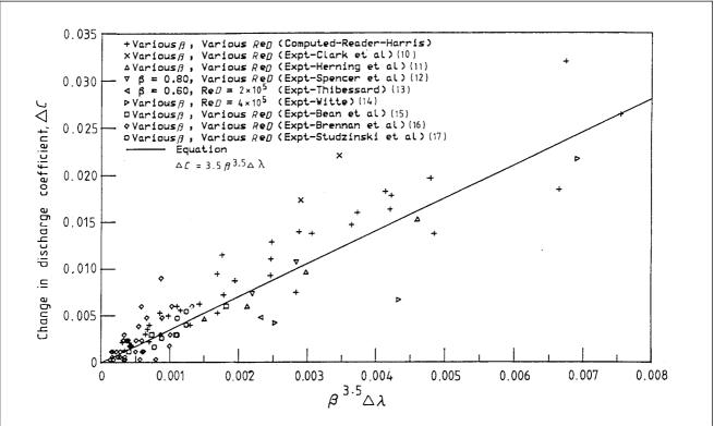
Figure 14. The effect of rough pipe on discharge coefficient
