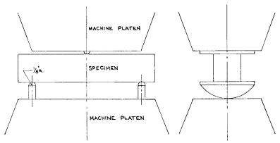
FIG. 2 Alternative Suggested Bearing Edge and Specimen Support
